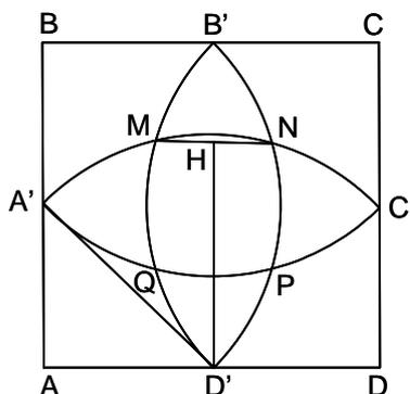
Los ángulos en  $D'$  valen:  $\widehat{AD'A'} = 45^\circ$ ,  $\widehat{A'D'M} = 30^\circ$ ,  $\widehat{MD'B'} = 15^\circ$ . El radio  $D'A' = r = \frac{a}{\sqrt{2}}$ ,
